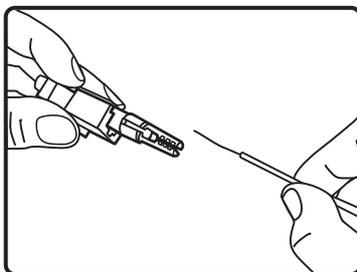
4. Retire a fibra óptica do conector.
