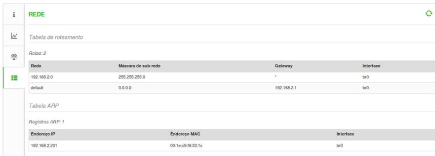
The screenshot shows the 'REDE' (Network) status page. It includes a sidebar with navigation icons and a main content area. The 'Tabela de roteamento' (Routing Table) is displayed, showing two routes. Below it, the 'Tabela ARP' (ARP Table) is shown with one entry.
